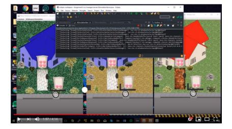
The sending client trace in atomic mode shows that it receives the inputstring, and then sends the command to the server without local processing. It then waits for the server to send the command back before processing.
